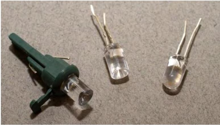
Examples of common white LEDs from holiday light strings. The two on the left are the “inverted cone” design which work best for structure lighting. The standard rounded end LED at right has a very directional beam, most suitable for headlights and spotlights. The LED at left is still in the original socket from the light string.
