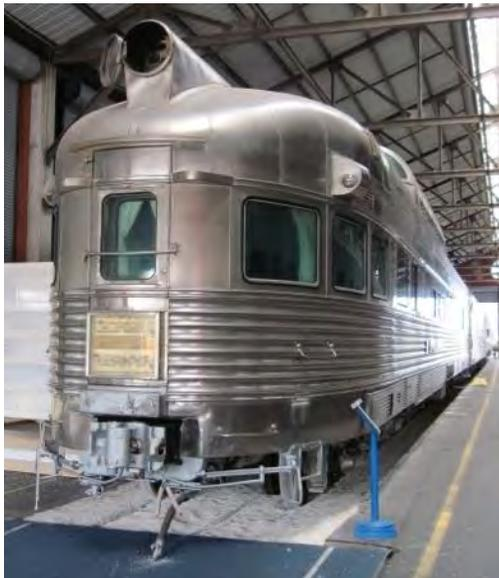
The “Silver Crescent” from the California Zephyr displayed in the train shed is an 85’ round end “Vista Dome” build by Budd in 1948. A “Vista Dome” graced the rear of every California Zephyr train; this car has logged over four million miles. The
