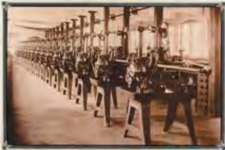
since I depicted them as being belt-driven. Note that the lathes and screw machines have pans for containing the cutting oils, while the presses have large drive wheels and parallel plates on which the dies were set. Here are some of the reference materials used, note that having people in the photos helps to provide a frame of
