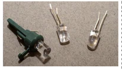
by a 12 volt DC power supply. It doesn't matter on which side (positive or negative) the current-limiting resistor is connected – just make sure to always use a current-limiting resistor, 1K current-limiting resistors are typically used
