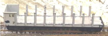
A razor saw was used to make the rough cuts, removing each panel next to the ribs (top). The cuts were made so they stopped above the floor of the car. To clean up the cuts (above), the inside of the panels was scribed and the snapped off and dressed out. The author made sure the floor was not damaged. Once painted (below), the finish car is ready for work.
