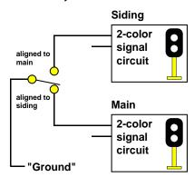
The first approach you may consider would be to connect the center pole of the contacts to "ground" and one input on each of the two block signals to the two positions of the contacts (see diagram on bottom of previous page).
