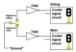
Note that the contact connections which control the red indication when the turnout is in each position is the opposite here. That's because the invertor changed the logic.
