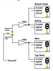
The two heads of the interlocking signal are connected just like the block signals. If we count all the NAND gates and invertors, we see we need four NAND gates and six invertors - and it just happens that four NAND gates are in one 7400 package and six invertors are in one 7404 package! But how to wire them easily? Next issue we will create a printed circuit board, and explain what "loose ends" need to be tied up to make this work reliably.
